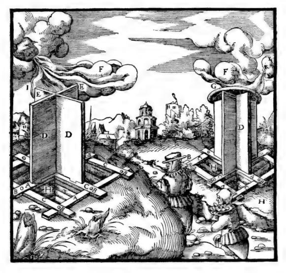
A-SILLS. B-POINTED STAKES. C-CROSS-BEAMS. D-UPRIGHT PLANKS. E-HOLLOWS. F-WINDS. G-COVERING DISC: H-SHAFTS. I-MACHINE WITHOUT A COVERING.
